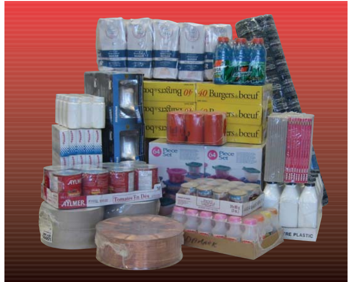
Below is a photo of a standard full enclosure style package. Note that we create the side seals by increasing the width of the film roll, letting it shrink to itself in the tunnel, then blowing it up upon itself, and finally we run it through the rollers.
