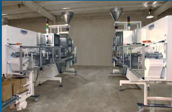
Dual-line, mirrored configuration capability allows one operator to control two machines.
