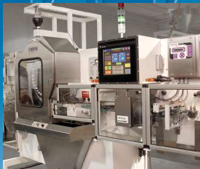
State-of-the-art Operator Interface, in-line metal detection, dust-reduction, and advanced safety guarding system
